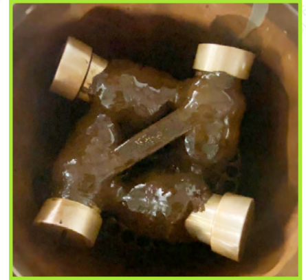
Magnetite collected on the external surface of the Rare Earth Magnetic Grate
